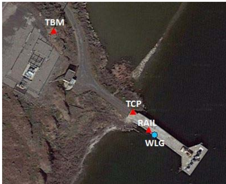
Figure 4. Water level gauge (WLG), RAIL point, temporary control point (TCP) and USACE temporary benchmark (TBM).
