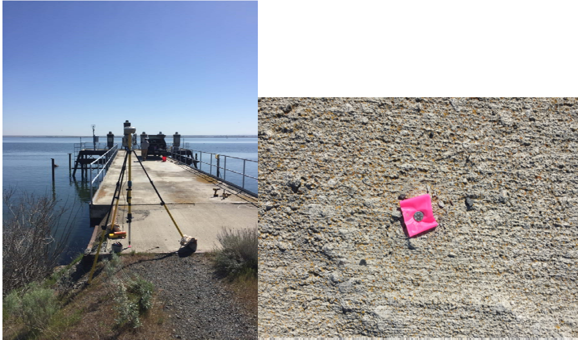
Figure 2. Temporary control point (TCP) establishment.
